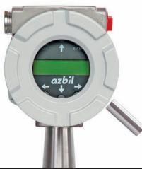
Azbil multivariable flowmeters utilize three primary sensing elements—a vortex shedding velocity sensor, an RTD temperature sensor, and a solid-state pressure transducer—to measure the mass flow rate of gases, liquids and steam.
