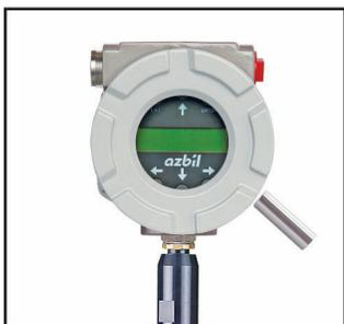
Azbil multivariable flowmeters utilize three primary sensing elements—a vortex shedding velocity sensor, an RTD temperature sensor, and a solid-state pressure transducer—to measure the mass flow rate of gases, liquids and steam. Because the AX23 is able to measure all process variables within a single device it provides exceptional accuracy, simplifies system design and reduces installation costs.
